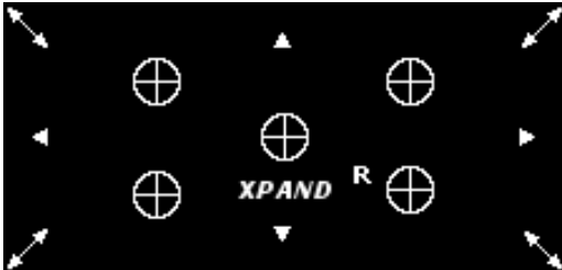
Figure 17: Central Image Scale/Zoom Adjustment using Screw H
